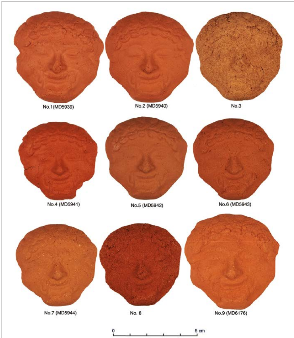
Fig. 15. Plasticity test: samples formed in plaster moulds and fired at 900°C in an oxidising atmosphere in a laboratory kiln (Digitizing M. Daszkiewicz, photos M. Baranowski)
