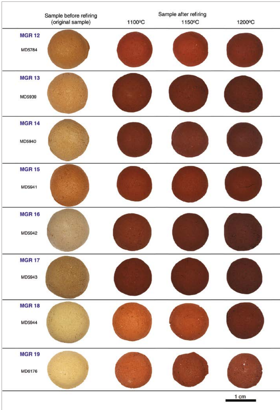
Fig. 16. Firing test results: briquettes made in porcelain moulds (Digitizing M. Daszkiewicz, macrophotos M. Baranowski)
